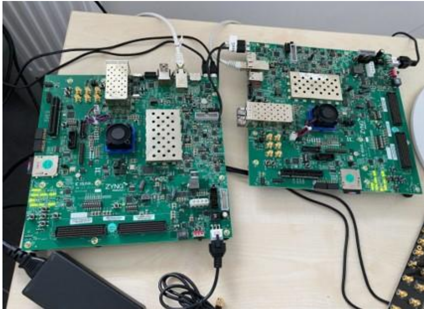
Fig 1. The FPGA are used to do post-processing to reduce the clock drifts of the quantum devices.
